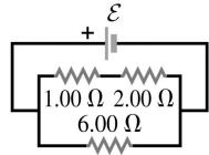
(b) (5) Calculate the equivalent resistance for all 3 resistors.
