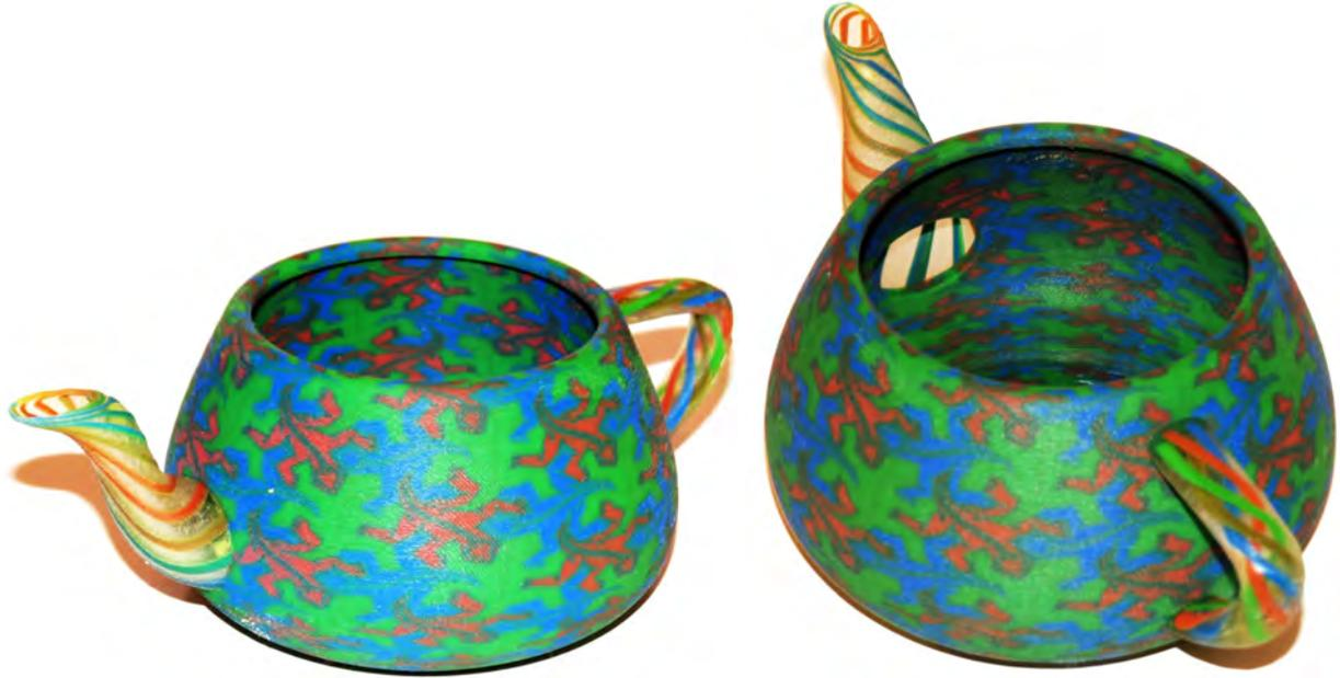
**Figure 4:** A fabricated object with graded materials based on a volumetric model of the Utah teapot. Printed courtesy of Stratasys Ltd.
