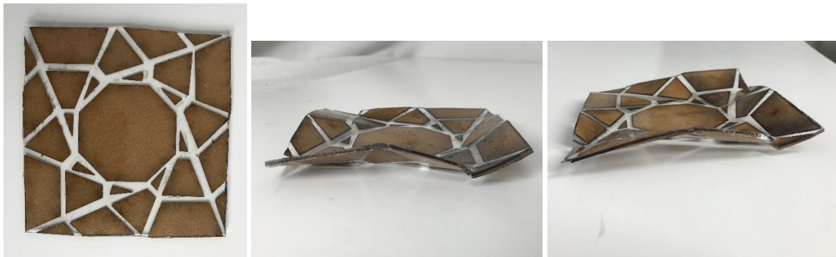
Figure 13: Full 1/16th MDF board laminated with SMP.
