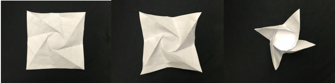
Figure 1: Paper model of the Pellegrino wraparound hub geometry.
