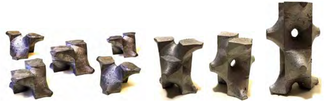
(a) Five views of a genus-0 space-filling tile. These tiles are cast in aluminum using 3D printed molds.
