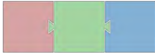
(b) A Geometrically Interlocking puzzle in 2-space. This puzzle cannot be assembled without lifting any piece into 3-space
