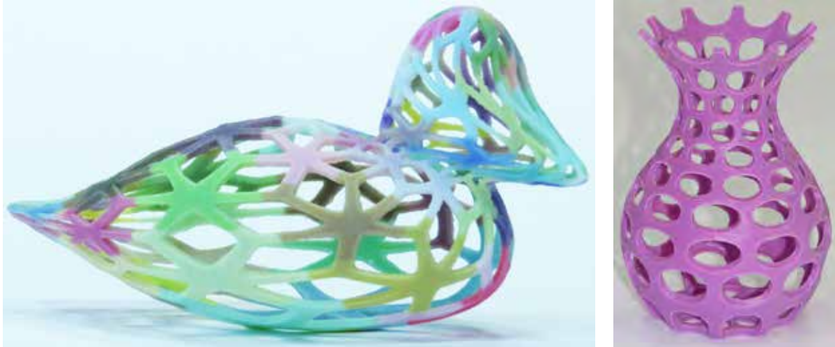
Figure 13: 3D printed samples. The duck is similar to the model in Figure 6 (a). The vase is the same geometry as in Figure 12. Printed on a J55 3D printer of Stratasys.
