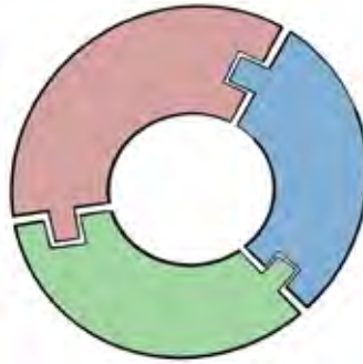
(c) A Geometrically Interlocking puzzle in 2-space that cannot be assembled without cutting one of pieces or lifting one of the pieces up into 3-space.
