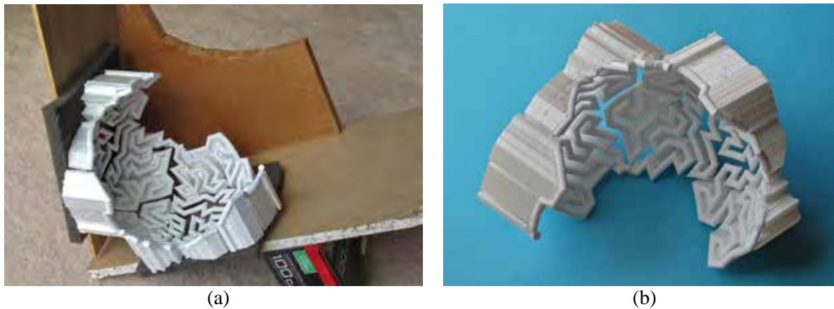
Figure 26: (a) Jig to hold two tetrants at the proper angle between them. (b) The resulting fused tetrant pair.
