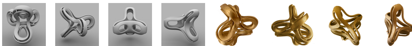
Figure 5: Models created in TopMod and 3D prints of the models For each sculpture, we took two photographs from slightly different point of views. The sculptures are photographed on a mirror. Background is eliminated. These shapes are made from ABS plastic and printed using a Fused Deposition Machine (FDM). They are later painted using an acrylic paint. The ribbon shape on the left is really a genus-1 surface, but, during the construction of this surface, genus changed several times.
