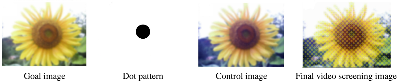
Figure 5: An example of using complementary colors. In this example, blue control image is created by eliminating its complementary color (in this case yellow).
