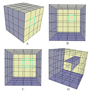
Figure 6 Screen capture of the mesh modelling system illustrating the use of the new display mode for modelling interior structures
