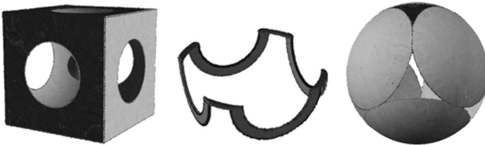
Figure 8. Some simple objects constructed by set-operations and painted by the implicit surface painter.
