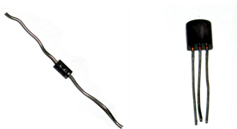
Figure 3. A real diode and transistor.
