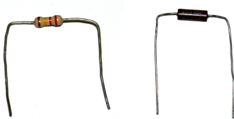
Figure 1. Photographs of a real resistance and inductance.
