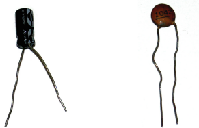
Figure 2. Photographs of two real capacitors.
