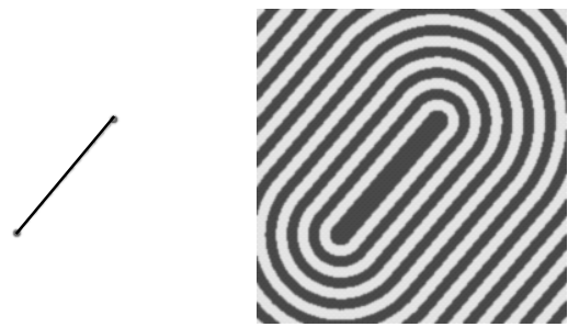
Fig. 2. Equidistant curves described by a distance function for an oriented line segment.
