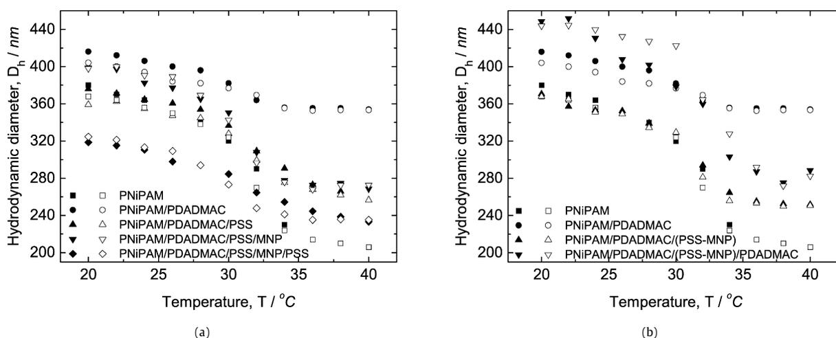
**Fig. 6.** The dependence of the hydrodynamic radius (as followed by DLS) of the hybrid core-shell PNIPAM microgel coated with polyelectrolytes and (a) MNP or (b) (PSS-MNP) as a function of temperature. Closed and open symbols represent the heating and the cooling cycle, respectively.
