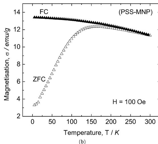
**Fig. 4.** (a) Magnetisation curves of positively charged MNP and negatively charged (PSS-MNP) exhibit zero coercivity and remanence indicating the superparamagnetic nature of both particles. (b) Temperature dependence of magnetisation of (PSS-MNP) at ZFC and FC conditions indicates the blocking temperature,  $T_{\text{B}} \sim 250$  K.
