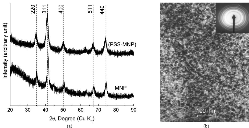
**Fig. 1.** (a) XRD patterns of MNP and (PSS-MNP) with characteristic peaks at  $2\theta \sim 35^\circ, 41^\circ, 50^\circ, 67^\circ$  and  $74^\circ$  confirm the presence of magnetite or maghemite. Vertical dotted line is only a guide to the eye. (b) TEM image shows (PSS-MNP) particles with a number-average size around 5 nm. The electron diffraction pattern is shown in the inset.
