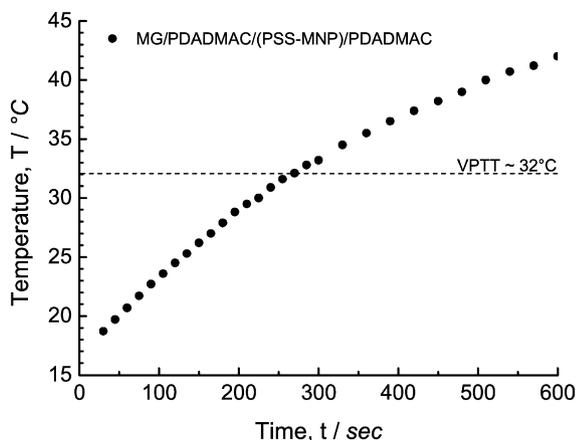
**Fig. 7.** Time-dependent temperature curve of MG/PDADMAC/(PSS-MNP)/PDADMAC microgels in a 200 kHz and  $3.8 \text{ kA m}^{-1}$  ac magnetic field. The corresponding SAR calculated is around  $600 \text{ W g}^{-1}$ .
