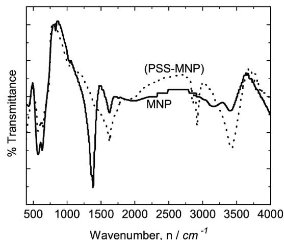
**Fig. 2.** FTIR spectra of positively charged MNP and negatively charged (PSS-MNP) provide evidence of the polyelectrolyte bound to the MNP. Additional peaks at 2930 and 2854  $\text{cm}^{-1}$ , and decrease in intensity at 588, 680 and 1380  $\text{cm}^{-1}$  supports the presence of PSS on (PSS-MNP) particles.
