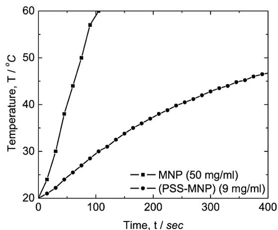
**Fig. 5.** Time-dependent temperature curves of positively charged MNP and negatively charged (PSS-MNP) in a 200 kHz and 3.8  $\text{kA m}^{-1}$  ac magnetic field show that sufficient heat is produced within a short time frame, even at low concentrations.
