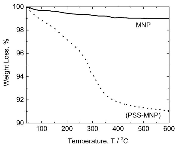
**Fig. 3.** TGA curves of positively charged MNP and negatively charged (PSS-MNP). The initial weight loss in MNP is due to evaporation of residual water, while the two-step weight loss in (PSS-MNP) is due to an initial loss of residual water followed by degradation of PSS.
