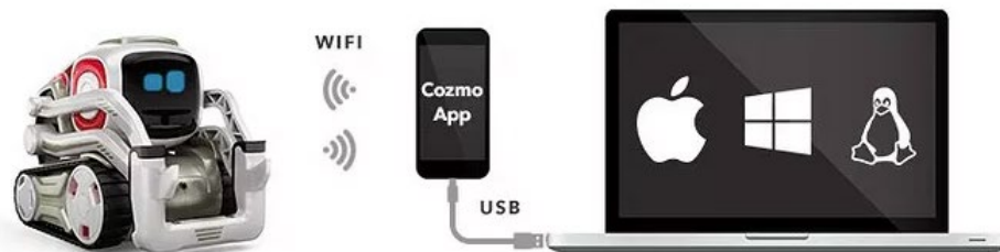
Hardware setup for the Cozmo SDK.
