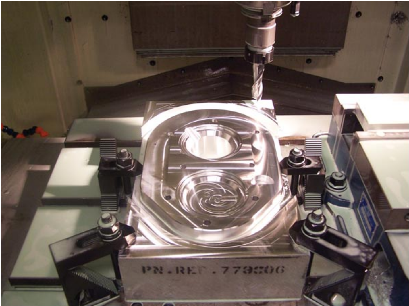
A large workpiece clamped to the table of a VMC using step clamps.
