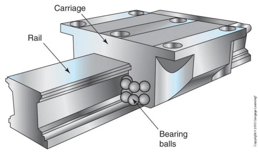
A linear guide assembly and its parts.
