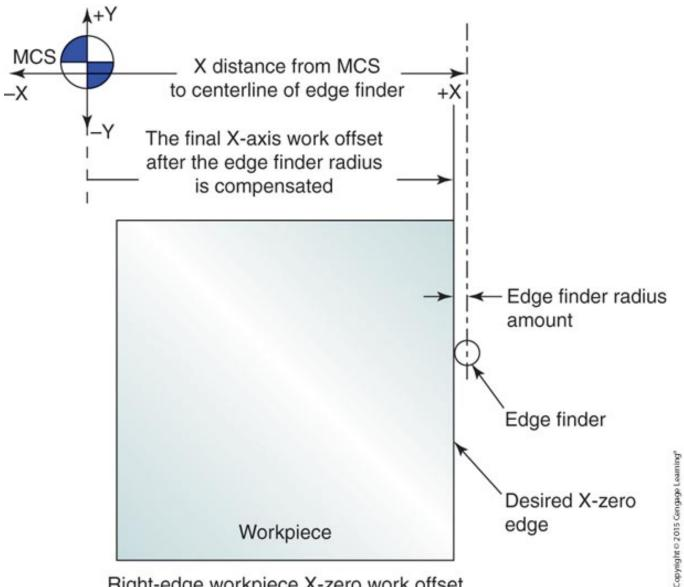
Right-edge workpiece X-zero work offset
