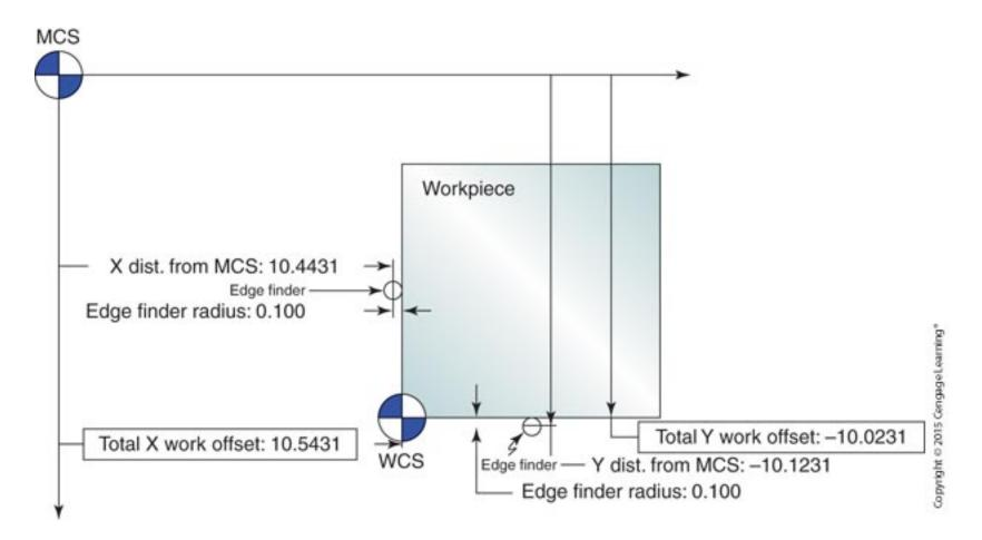
A dimensioned example of how a work offset is derived for a workpiece having the origin in the front left corner.
