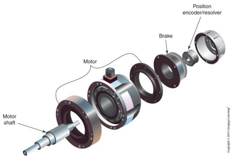
The parts of a servo motor.
