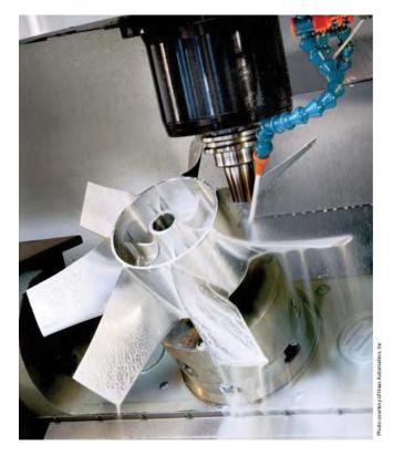
CNC milling machines can produce complex part surfaces that would be virtually impossible to produce with manual milling machines.
