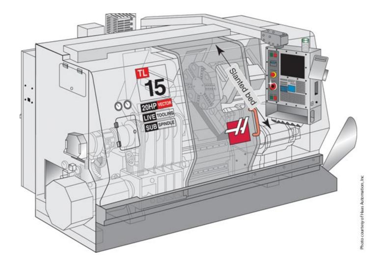
A slant-bed turning center has an inclined bed.
