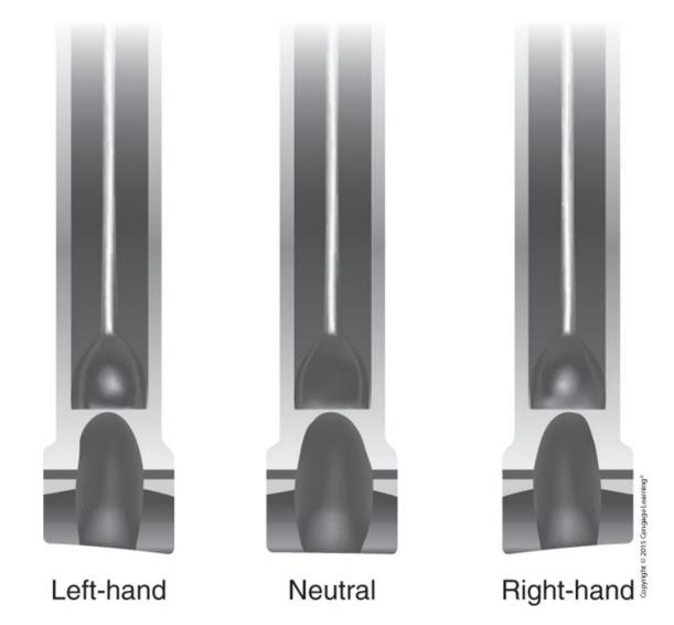
Cutoff inserts are available with a biased cutting edge to minimize burrs on the part being cut off.
