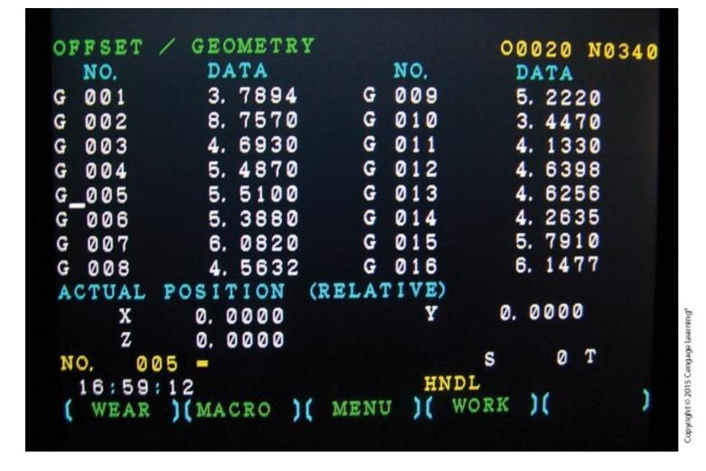
A typical milling geometry offset page on the machine display screen. These numbers reflect the tool length from gage line to the tool tip in its original and unworn state.
