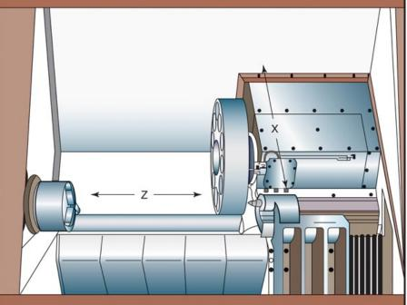
The coordinate system for CNC turning and the relationship of the axes.
