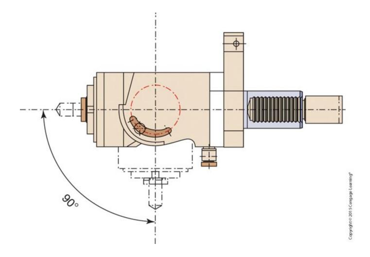
An adjustable angle-head live tooling attachment allows angular milling to be performed on the turning center.
