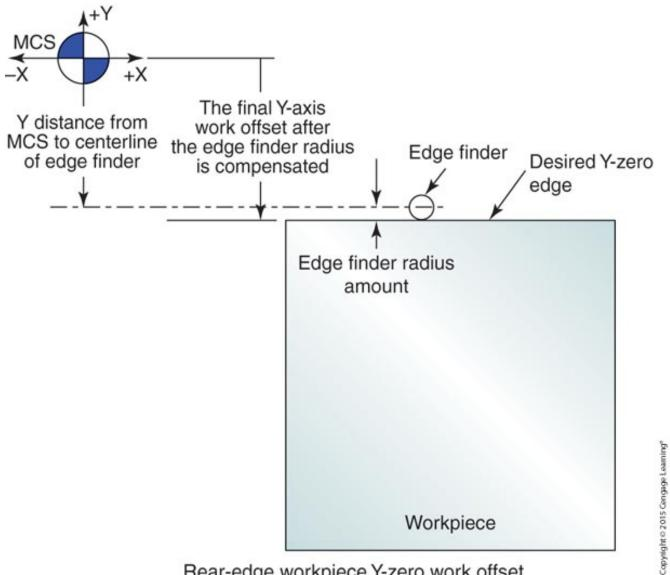
Rear-edge workpiece Y-zero work offset
