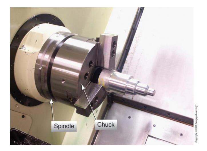
A three-jaw power-actuated chuck in a CNC turning center. This setup is using soft jaws that were machined to match the outside diameter of the workpiece.
