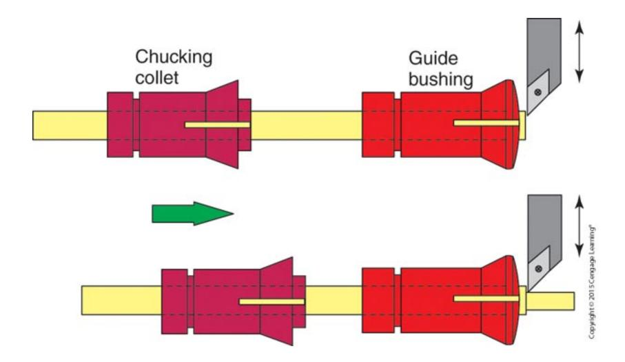
A Swiss turning machine moves the entire workpiece in the Z-axis instead of moving the cutting tool.
