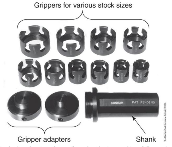
A gripping-ring-type bar puller grips the bar end by sliding a ring of spring-steel teeth over the perimeter of the bar.
