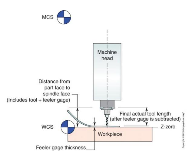
A VMC Z-axis can be used to measure tool length. The length offset is found by touching the tool tip off of the work Z-zero surface with a feeler gage and then subtracting the feeler gage thickness. The objective is to determine the dimension labeled "Final actual tool length."
