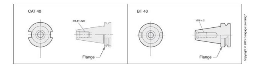
A CAT holder and a BT holder. Notice the difference in the size of the flanges and the location of the grooves.
