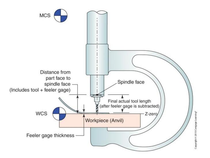
The way a VMC Z-axis can be used to measure tool length can be compared to the way a micrometer measures.
