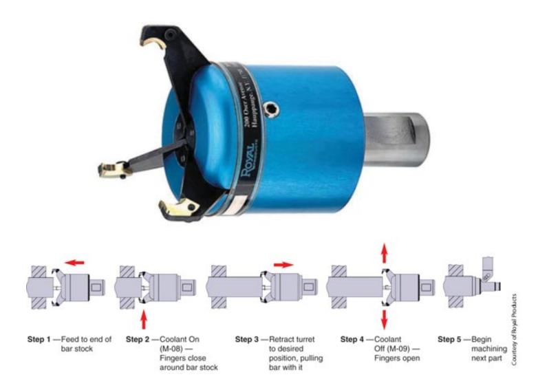
This coolant-actuated bar puller's jaws grip the stock using the hydraulic pressure of the machine's coolant system.
