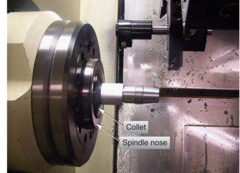
A CNC turning center using a collet for workholding.
