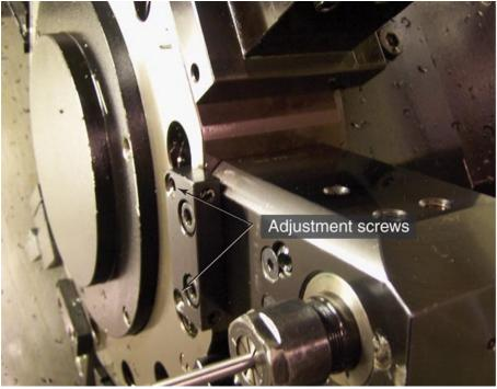
Adjustment screws for squaring a holemaking tool holder.
