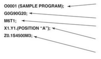
Program number and (operator label). Since this label is within parentheses, it is not read by the machine, only by the operator.
