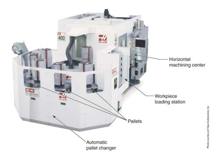
This machining center has an APC that uses six pallets. The machine can be programmed to load any of the pallets automatically. Work is loaded on each pallet at the station on the right side of the APC.
