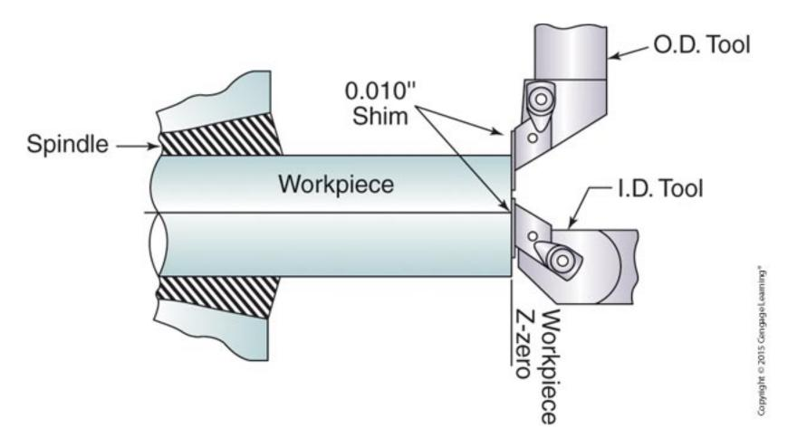
Method for setting tools off the part face of Z-zero with a 0.010"-thick feeler gage. While in this position the tool's position can be set as positive 0.010" in the Z-axis.
