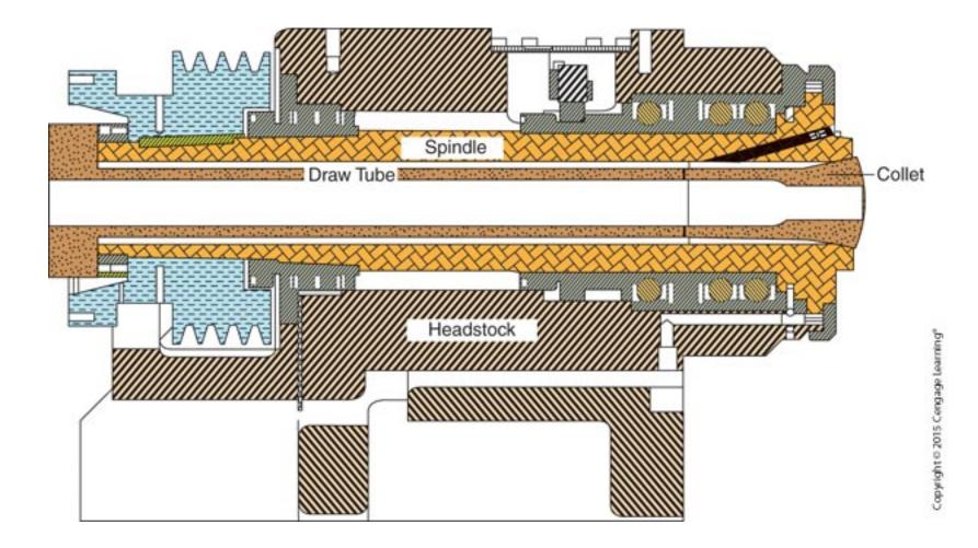
A turning center drawtube and collet assembly within a machine spindle.
