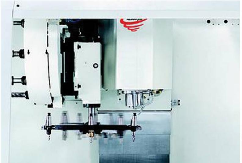
The swing-arm-type ATC changes tools much faster than the carousel-type ATC.
