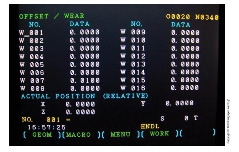
A typical milling wear offset page on the machine display screen. The number that will be entered into the wear offset will be an incremental adjustment from a baseline of zero tool length wear.
