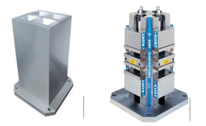
The tombstone tower in (A) can be machined as needed for mounting work or other workholding devices. The tombstone tower in (B) has four integrated vises, one on each of the four sides of the tower.
