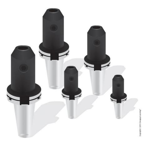
National Machine Tool Builder (NMTB) toolholders in 30, 35, 40, 45, and 50 size tapers. Retention knobs thread into tapered toolholders to secure the holder in the machine spindle.
