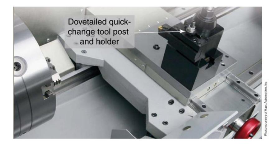
Quick-change toolholders used on a CNC lathe.
