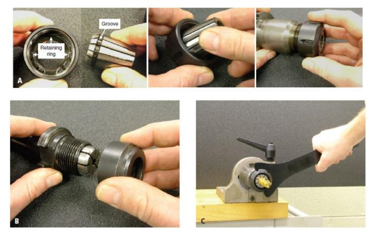
(A) The groove on an ER collet snaps into a retaining ring in the threaded cap and the cap is then threaded into the collet chuck. (B) DA collets slip into the chuck and then the cap is threaded onto the chuck. (C) The toolholder is then mounted in a bench-top clamping device, the tool is inserted in the collet, and the cap is tightened.
