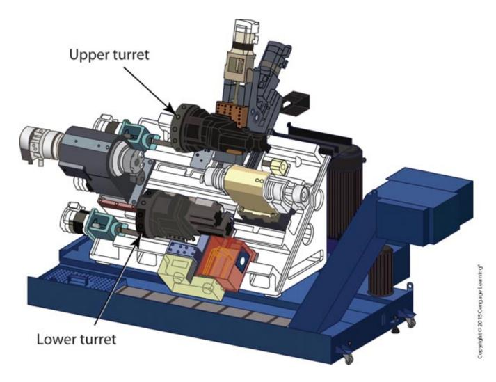
A twin turret machine can move both turrets independently for machining.
