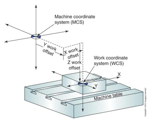
Workpiece offset, or workshift, is the distance from the MCS origin to the desired location of the WCS origin.
