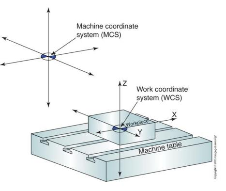
The relationship of the machine coordinate system (MCS) to the work coordinate system (WCS).
