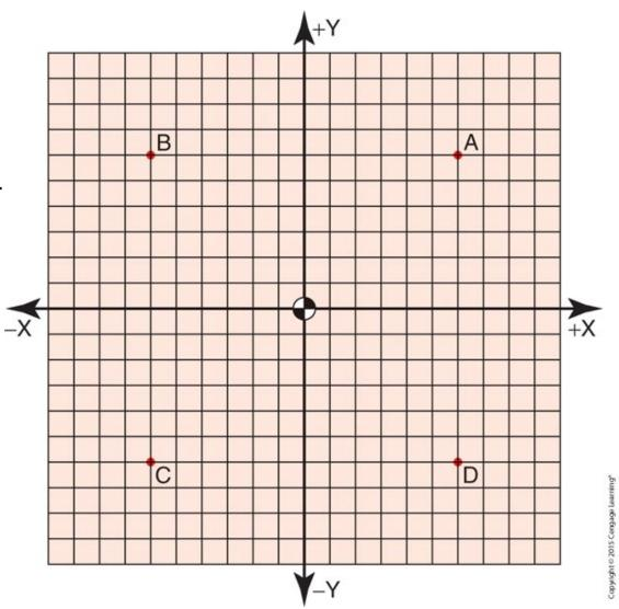
Assume that each block on the grid equals 1". Using the incremental programming method, assuming the cutting tool is already at position A, the coordinates for each following location are: (B) X-12.0 Y0; (C) X0.0 Y-12; (D) X12.0 Y0.0
