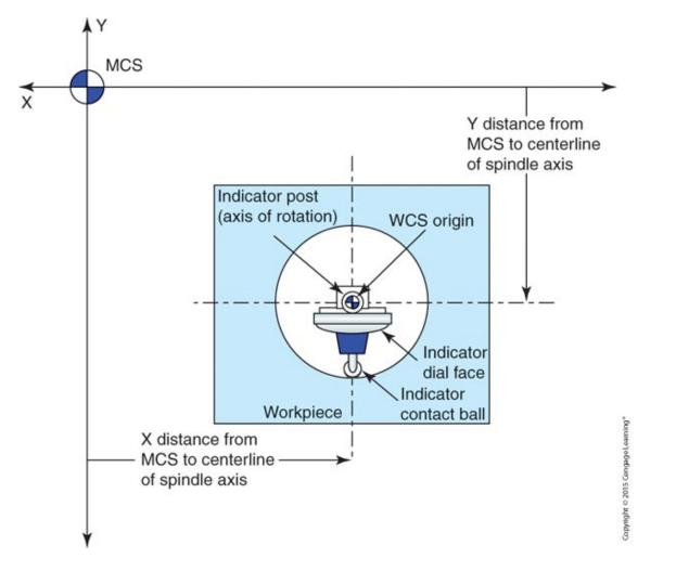
This top view shows that when a hole center is to be used as the X/Y location of the work origin, the hole center can be found by sweeping with a dial indicator. This aligns the spindle centerline with the hole centerline.
