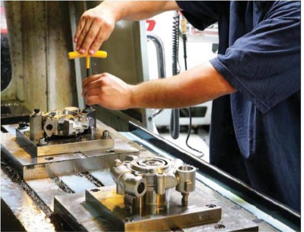
A custom fixture designed and built to hold an oddly shaped pump housing.
