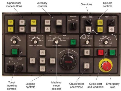
The parts of a turning center control panel.
