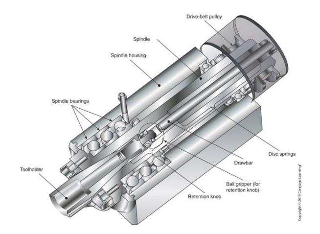
A cutaway view showing the many parts of a milling spindle. Notice how the ball gripper mechanism at the end of the drawbar grasps the retention knob. Spring tension from a series of disc springs pulls on the drawbar to secure the toolholder taper.
