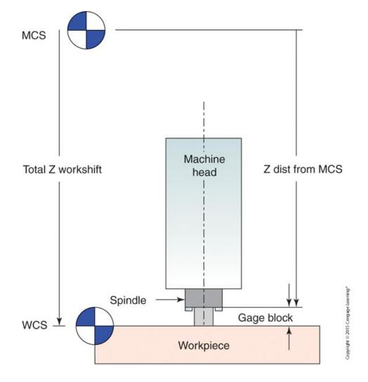
This front view shows a VMC spindle face and a gage block being used to determine the Z-axis work offset. Note the relationship of the MCS to the WCS.
