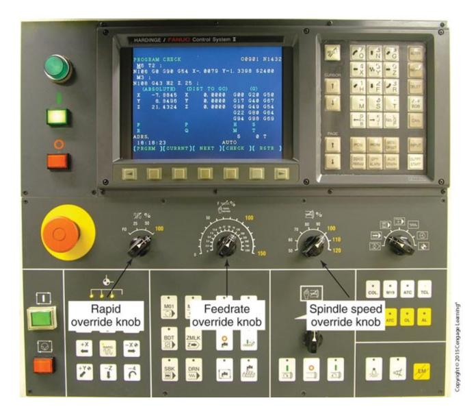
A spindle speed, feed rate, and rapid override control.
