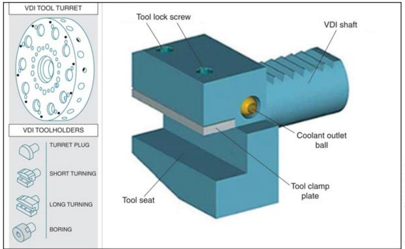
A VDI toolholding adapter mounts to the turret with a VDI shank. The adapter is drawn tight to the turret with the serrated teeth.
