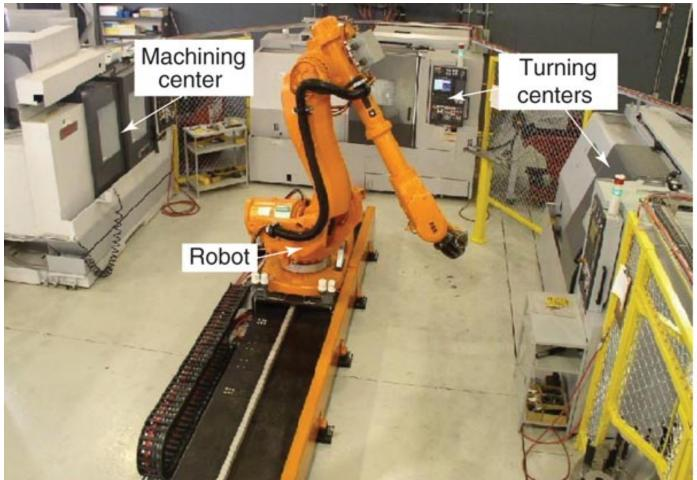
A robotic manufacturing cell can enhance productivity by minimizing operator intervention. The workpiece is transferred between machines by the robot. A specialized mill/turn machine that can perform heavy milling and turning operations.
