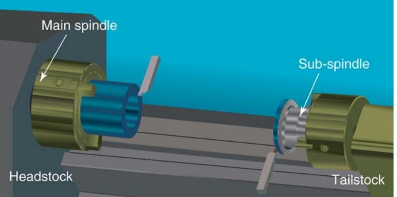
A sub-spindle opposes the machine's main spindle. The workpiece can be transferred from the main spindle to the sub-spindle so that the backside of the workpiece can be machined.
