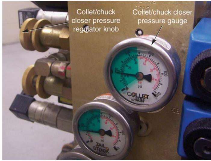
A picture of a turning center hydraulic regulator and gauge for adjusting collet or chuck clamping pressure.
