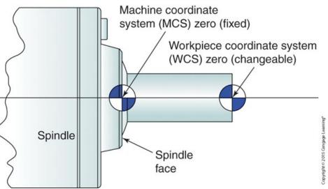
The relationship of the machine coordinate system (MCS) to the established work coordinate system (WCS).
