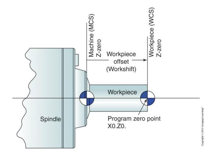
Workpiece offset is the Z-axis distance from the MCS zero to the WCS zero. The X-axis offset should remain zero since the spindle and workpiece share the same center line.
