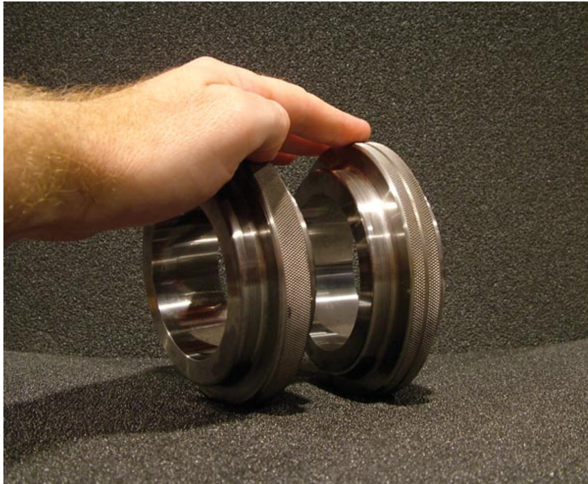
FIGURE 2.4.12 Go and no-go plain ring gages. Note the groove around the circumference to identify the no-go gauge.
