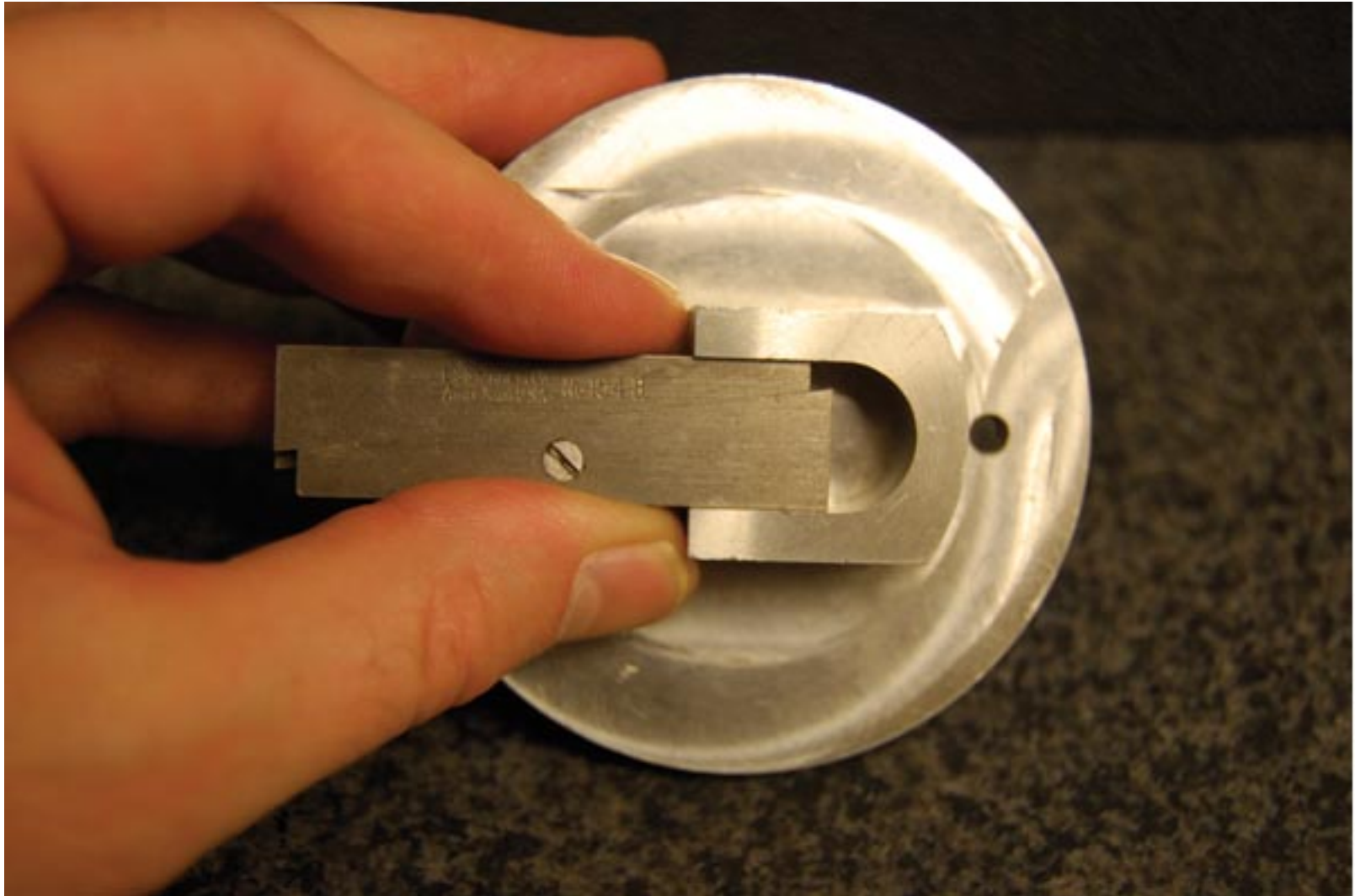
FIGURE 2.4.86 Measuring a slot width with an adjustable parallel.
