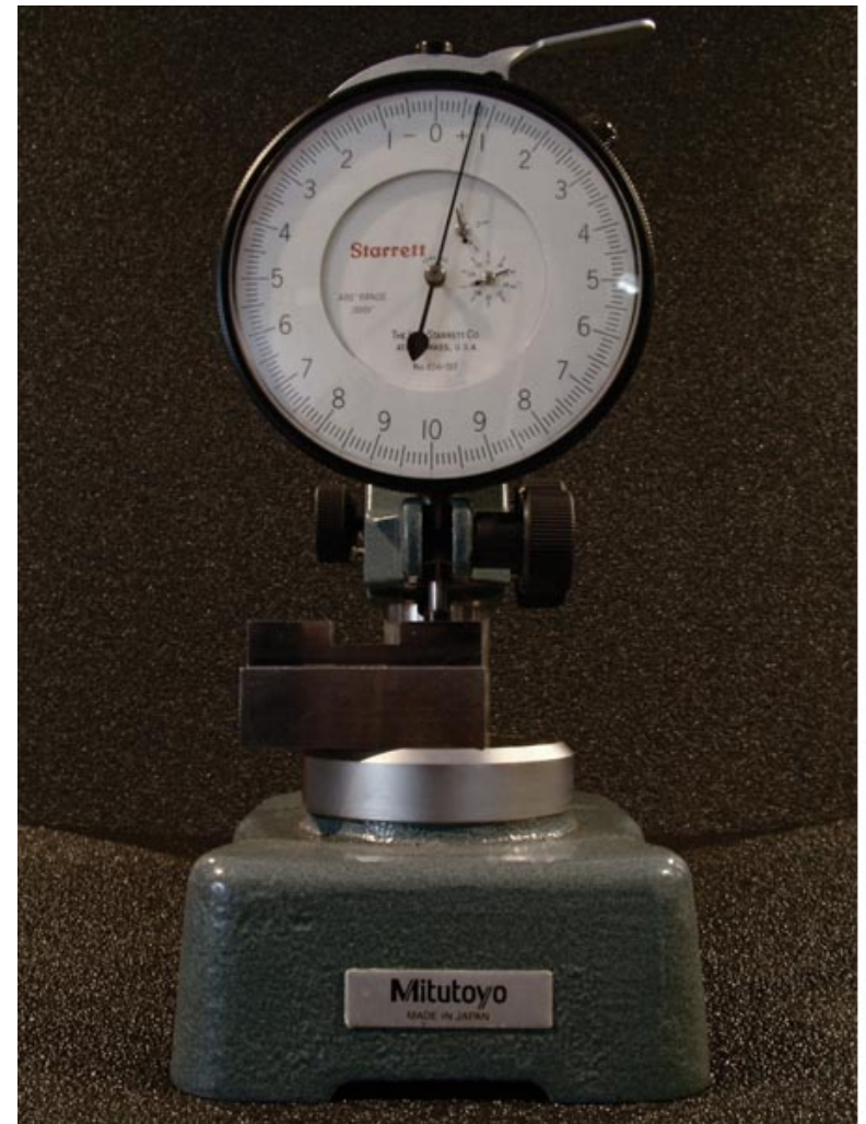
FIGURE 2.4.92 (A) Mastering a dial indicator with a gage block build. (B) Checking a measurement with the drop gage. Note the lever that can be used to raise and lower the indicator contact.
