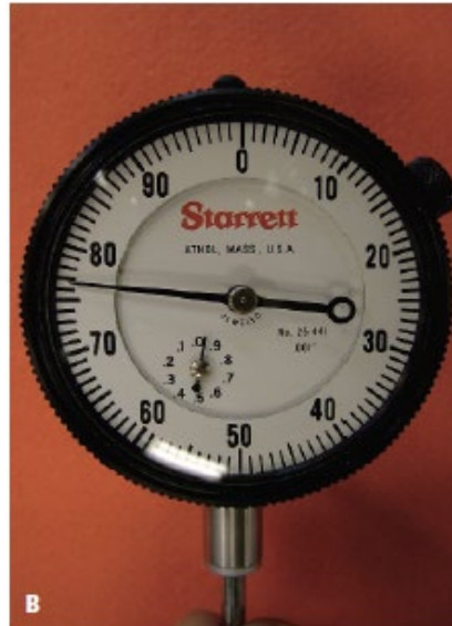
FIGURE 2.4.88 (A) A balanced-type dial indicator face with 0.0005" graduations. (B) A continuous-type dial indicator face with 0.001" graduations. (C) A continuous face with 0.001" graduations and a second set of numbers. Note the counter-dial on the continuous face dials to keep track of the revolutions of the main needle.
