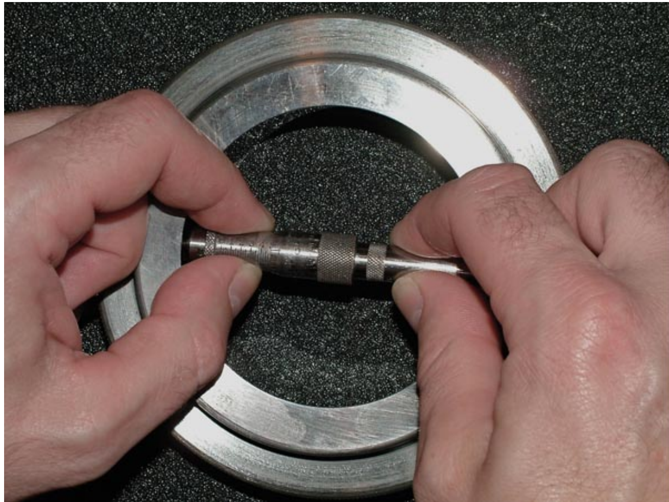
FIGURE 2.4.66 Taking a measurement using an inside micrometer.
