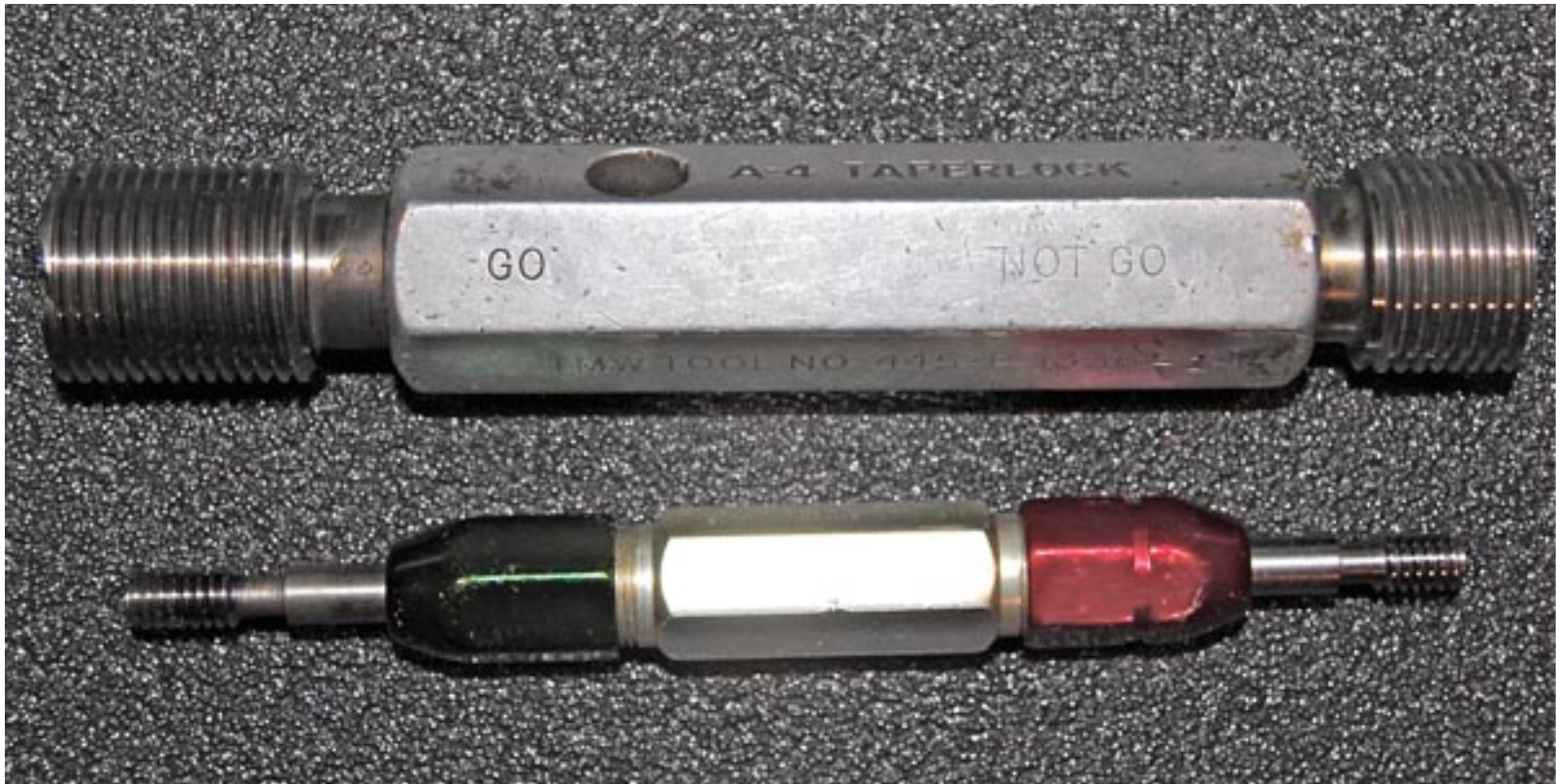
FIGURE 2.4.9 Two typical go/no-go thread plug gages. The go member is either marked as green or is longer than the no-go member, just like a plain plug gage.
