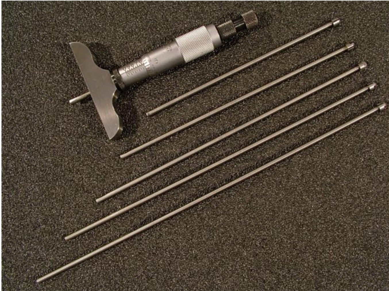
FIGURE 2.4.69 A depth micrometer with rods for different size ranges.
