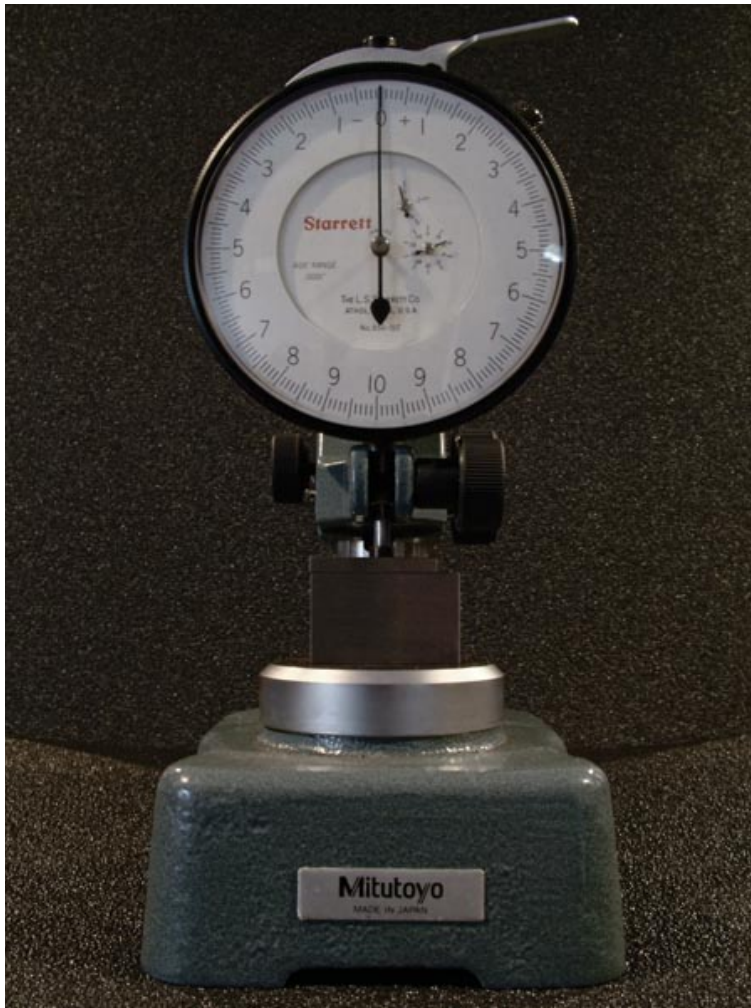
FIGURE 2.4.92 (A) Mastering a dial indicator with a gage block build. (B) Checking a measurement with the drop gage. Note the lever that can be used to raise and lower the indicator contact.
