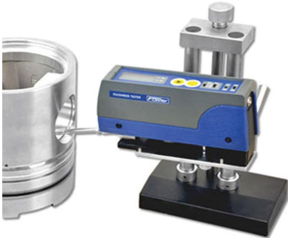
FIGURE 2.4.108 A portable profilometer measuring the surface finish of the hole in a machined component.
