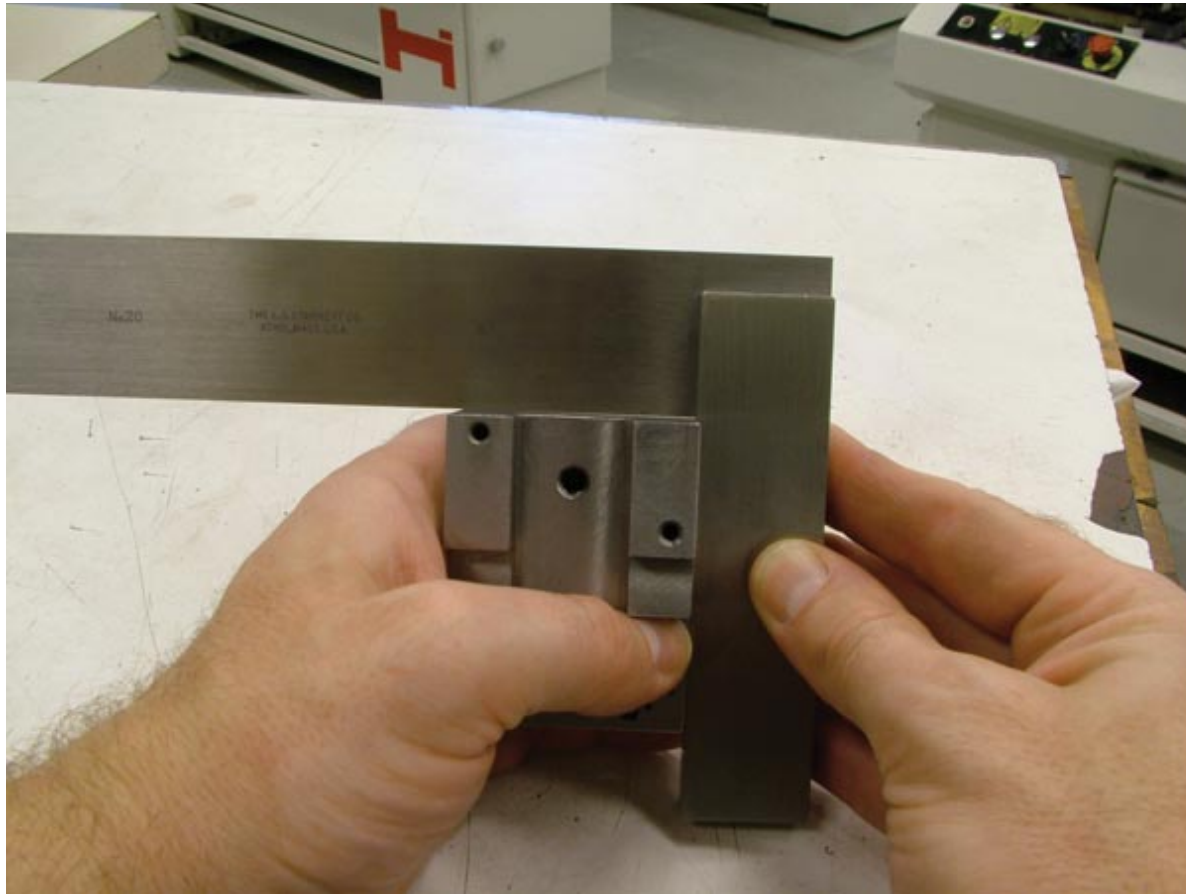
FIGURE 2.4.20 Checking two surfaces for square (perpendicularity) with a solid square. The light showing between the part and the blade at the inner corner indicates the two surfaces are “out of square.”
