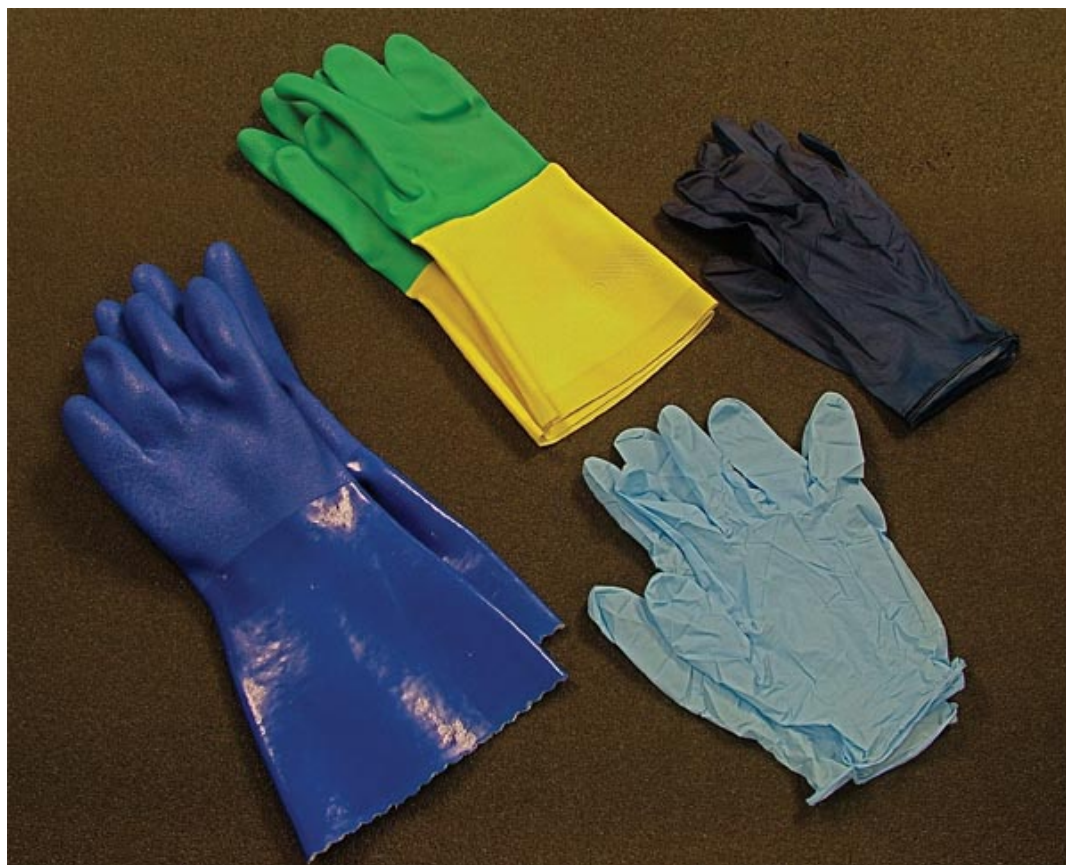
FIGURE 2.1.8 Different gloves are available for different uses. Note the different lengths. When handling chemicals, always follow the chemical manufacturer's recommendation for the proper type of glove.
