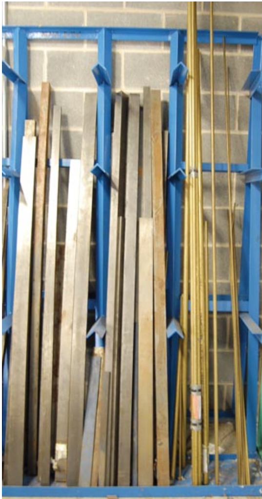
FIGURE 2.1.9 Store material in proper racks like these for safety. Don't stack it on the floor, workbenches, or machinery.
