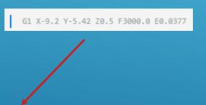
▶ Interpretation: move towards X=-9.2, Y=-5.42, and Z=0.5 in a straight line at a feed rate of 3000.0 while extruding 0.0377 mm of material.
