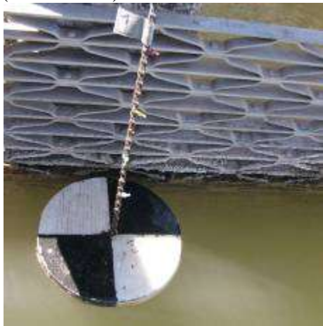
Photo C4. The Secchi disk that was used to measure visibility and in the second photo an intern, Army Specialist Justin King, practicing the Secchi disk measurement in Cantonment A Pond (Reservoir 3).
