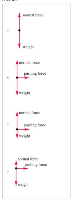
If you were actually going to solve this problem rather than just draw the free-body diagram, you would need to define the coordinate system. Choose the position of the piano as the origin. In this case it is simplest to let the *y* axis point vertically upward and the *x* axis point horizontally to the right, in the direction of the acceleration.
