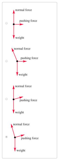
In working problems like this one that involve an incline, it is most often easiest to select a coordinate system that is not vertical and horizontal. Instead, choose the *x* axis so that it is parallel to the incline and choose the *y* axis so that it is perpendicular to the incline.
