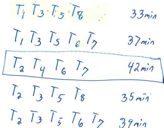
Critical path is  $T_2 \rightarrow T_4 \rightarrow T_6 \rightarrow T_7$
