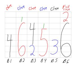
First-fit Algorithm (FF): Put items into the first already open bin that has space for it. If no open bin has space, open a new bin.
