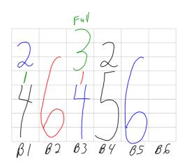
**Best-fit Algorithm (BF):** Put items into an already open bin that has the least space for it. If no open bin has space, open a new bin.
