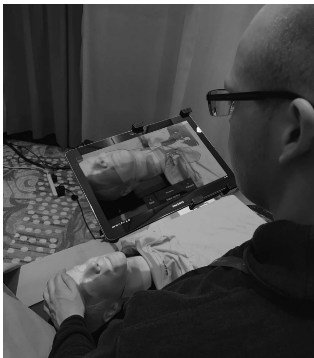
FIGURE 1. Prototype of our AR telementoring system, used here with a cricothyroidotomy simulator. The trainee looks at the patient simulator through the AR display that superimposes onto the simulator a visualization of future steps of the procedure, here the initial incision.
