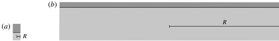
FIGURE 10. To-scale side view of the two reduction cell configurations studied in the article. (a) Small experimental cell with radius  $R = 0.035$  m used for the validation of the theory. (b) Large industrial-scale cell (in this plot  $R = 1$  m).
