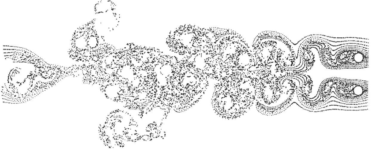
Figure 1: Streaklines about two cylinders, g^* = 2.5 .
