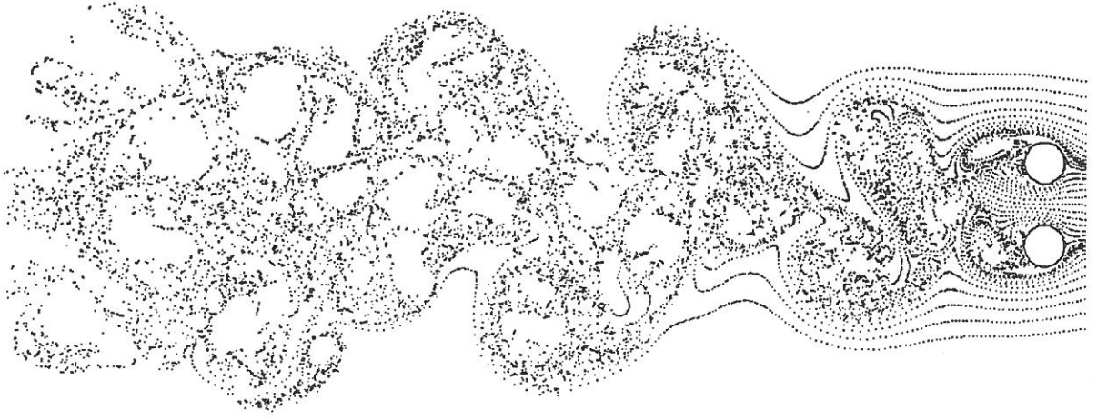
Figure 2: Streaklines about two cylinders, g^* = 1 .
