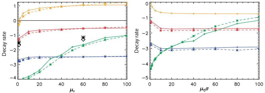
Figure 13. Growth rates for the MND flow driven dynamo against  $\mu_r$  (left panel) and against  $\mu_0\sigma$  (right panel). Solid curves denote data obtained from the FV/BEM scheme, dashed curves denote the results from the SFEMaNS scheme. The green, blue, red, yellow colors denote the cases  $Rm=0, 30, 50, 70$ . The black stars in the left panel show the results for the SMND flow at  $Rm=50$  (see text) as reported in table 3.
