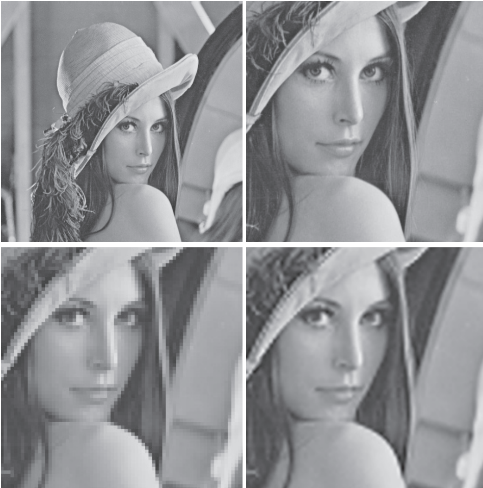
FIG. 10. Lena test: Original image and zoomed part (top); downsampled (bottom left); and s1 reconstruction (bottom right).
