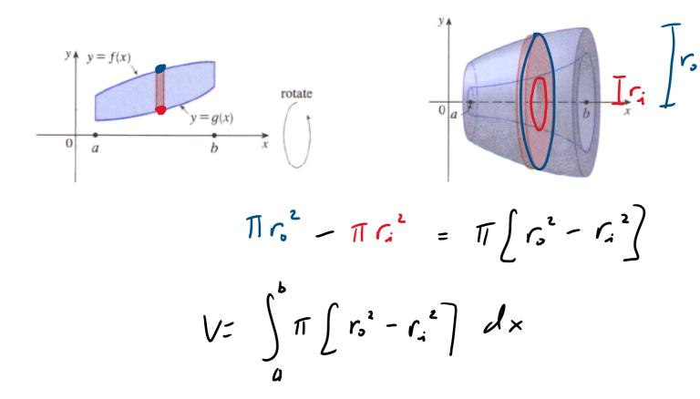
Example: Set up the integral(s) that would give the volume of the solid obtained by rotating the region bounded by the given curves around x-axis.
