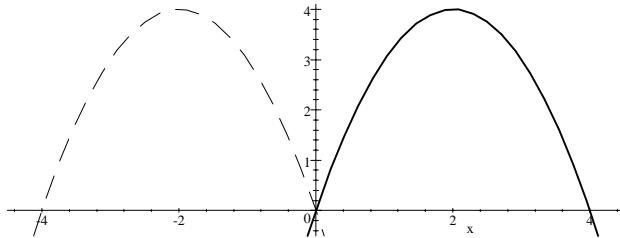
$$V = \int_0^4 2\pi x h dx = \int_0^4 2\pi x[x(4-x)] dx = \int_0^4 2\pi[4x^2 - x^3] dx = 2\pi \left[ 4\frac{x^3}{3} - \frac{x^4}{4} \right]_0^4 \\ = 512\pi \left[ \frac{1}{3} - \frac{1}{4} \right] = \frac{512}{12}\pi = \frac{128}{3}\pi \text{ (a)}$$
